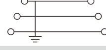
2.5mm 2 三层斜面等电位接地端子 Tripe level angled type ground terminal block with equipotential bonder
