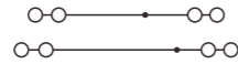
斜面双层八线接线端子 Double level angled type terminal block 8-wire
