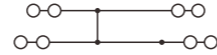
斜面双层八线等电位接线端子 Double level angled type terminal block with equipotential bond 8-wire
