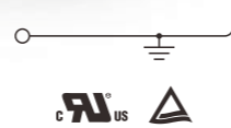
2.5mm² 一针一线插拔式接地端子 1-1 Feed Through Ground Pluggable Terminal Block
