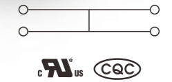
254系列两进两出带固定器正面接线端子 254 Series 2-2 Feed Through Terminal Block With Fixing Flanges of Front-entry
