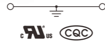
254系列一进一出正面接地端子(小导轨35) 254 Series 1-1 Feed Through Ground Terminal Block of Front-entry(SP35X7.5)
